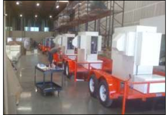
Solar powered, mobile, water purification units being manufactured at Mark's plant
